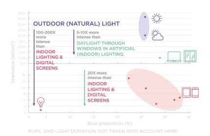
**Figure 2:** Comparison of light levels, natural light vs. common artificial lights
