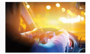
**4D COMPONENTS:** Flashing lights, point-like sources, high contrast of luminances, high blue component in LED headlights
